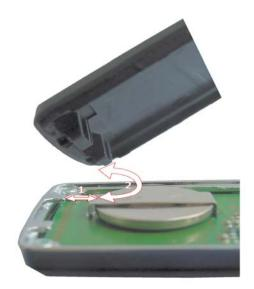
Lift the cover slightly and slide the cover backwards so that the brackets are released from the top. (1)
